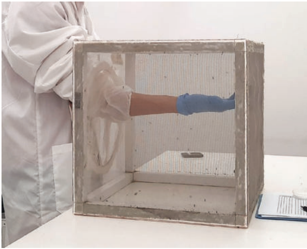
Fig. 4. Arm-in-cage test being conducted in a 0.064 m 3 cabin. A study participant exposing a full forearm (surface area: 600 cm 2 ).
