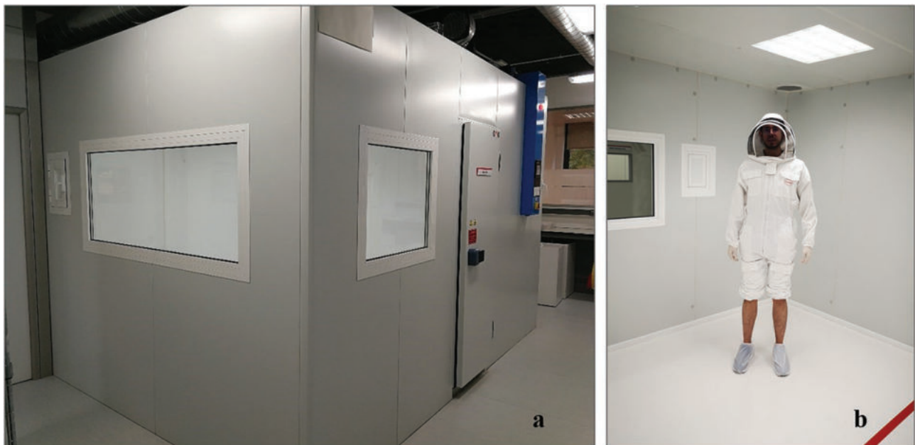
Fig. 3. (a) Outside view of the 30 m 3 testing room at Henkel’s R&D Insect Control Laboratory; (b) participant wearing a protective suit while inside the testing room.
